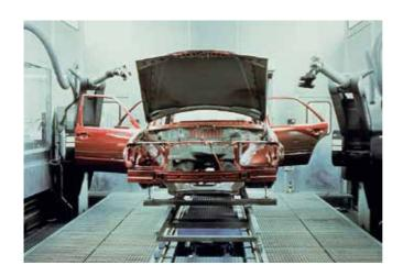
reduced, because these substances are blamed for causing summer smog and other nuisances. 2K acrylic paints were developed further into low-solvent high-solids, i.e. paints with a lower solvent content and a higher share of solid particles. The mid-eighties also saw the launch of the first waterborne paints, which have since become the standard type of paint both in OEM coating and refinishing.
